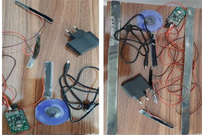
Figure 4 - Electronic circuit, bending sensors and pressure sensors
