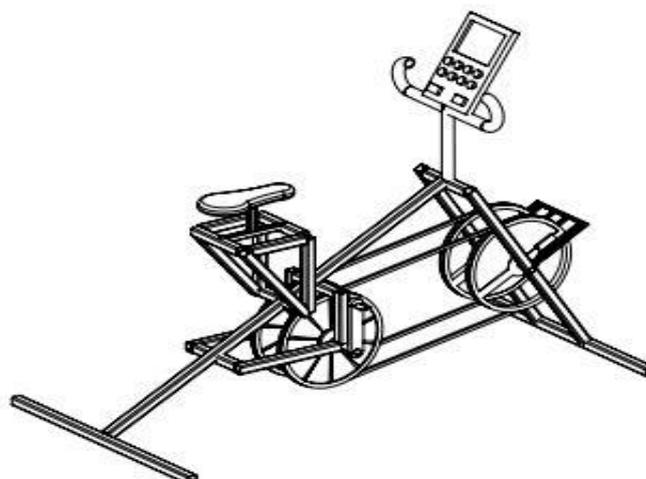
**Figure 3.** Overall look of Magnetic Stationary Bike with Simultaneous Different Workloads for each Foot
