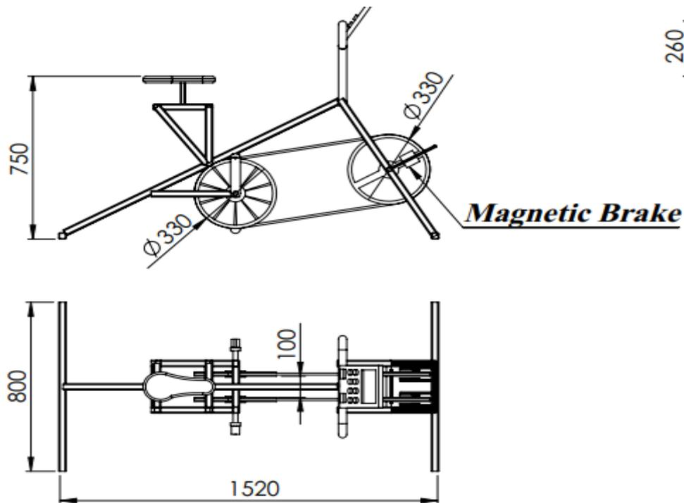
**Figure 4.** Location of the brakes and shows the dimensions of the pedals, wheels and the location of the brakes and symmetrical design of the wheels to apply different brakes on each of the pedals.
