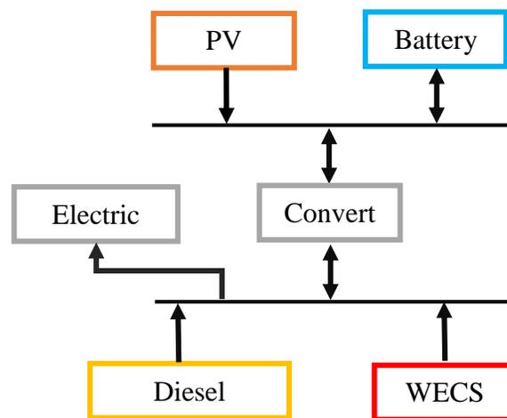
Figure 1. Energy flow diagram of the system.
