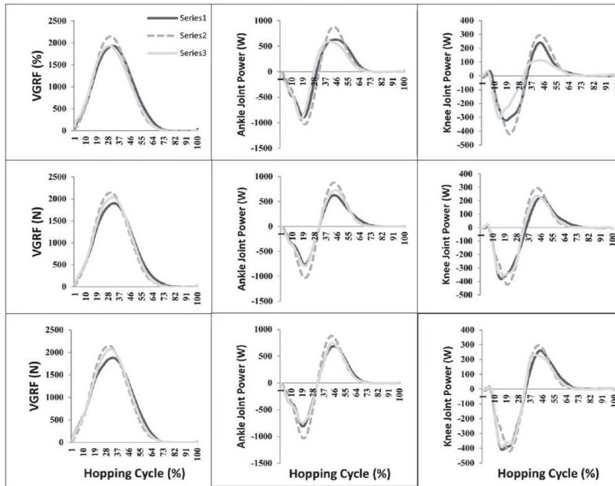
**Figure 3.** Vertical ground reaction force and mechanical power of ankle and knee joint on 300 kN/m (a), 400 kN/m (b) and 500 kN/m (c) surfaces in comparison to force plate (dotted line) before (dark line) and after (bright line) familiarity to surfaces.
