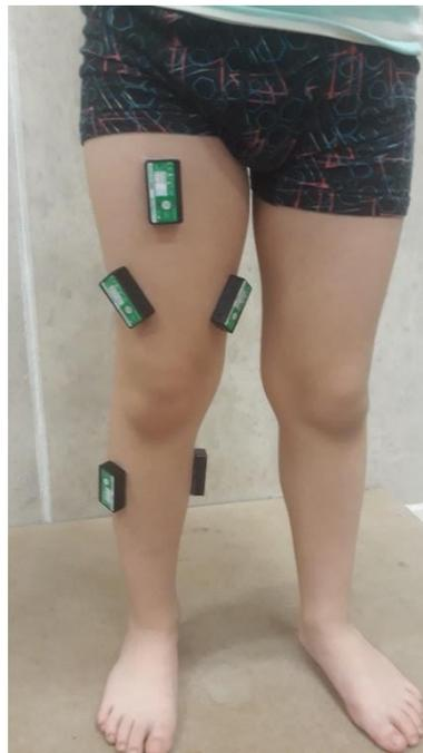
**Figure 1:** Electrodes positions in according to SENIAM recommendation
