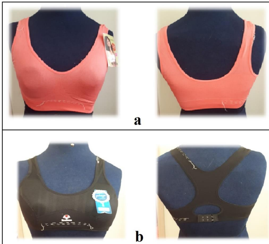
Figure 2. Samples prepared to evaluate movement comfort: a) non-padded seamless sports bra that had only a seam on top of the shoulders (sample SB1), b) spongy sports bra with some components (sample SB2)
