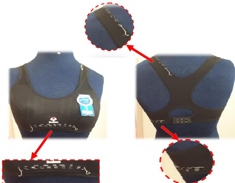
Figure 3. Selected areas for sewing metal thread to a sports bra
