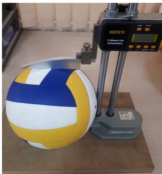
Figure 1. The caliper used to measure the diameter of sample balls
