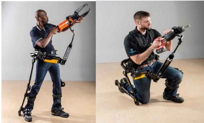
**Figure 10.** Lockheed Martin-Designed Fortis Exoskeleton for Workers Using Heavy Tools (20)
