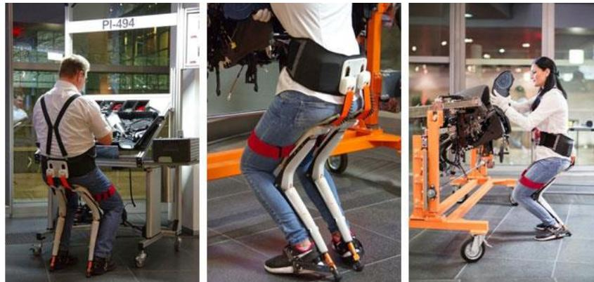
**Figure 9.** Noonee AG-Designed Chairless Exoskeleton for Production Line Workers Who Toil in Poor Conditions (19)
