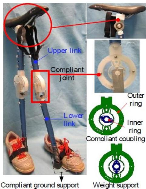
**Figure 2.** External Skeleton Supporting Body Weight, The Seat and Knee Components In Two Positions (10)
