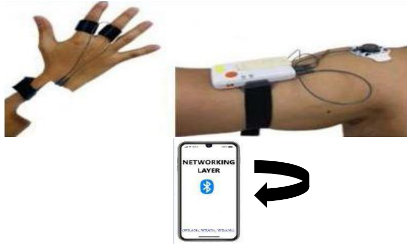
Figure 1. Multiple sensors located for measurement and evaluation of hand vibrations.
