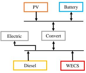
Figure 1. Energy flow diagram of the system.
